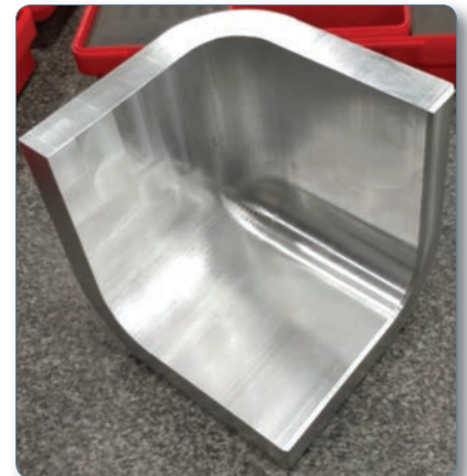
Relief Cut Fill Piece Fit Up Example (Above) Machined Corner Example (Right)
