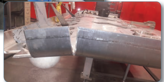
Examples of Relief Cuts from a 5/8-inch Thick Shell
