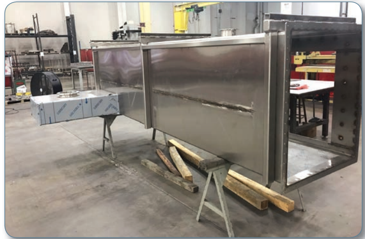
Example of Welded-On Stiffener Structure
