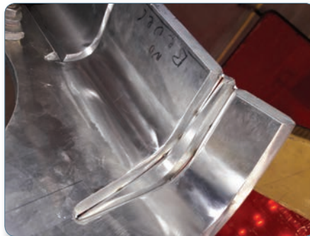
Relief Cut Fill Piece Fit Up Example (Above) Machined Corner Example (Right)
