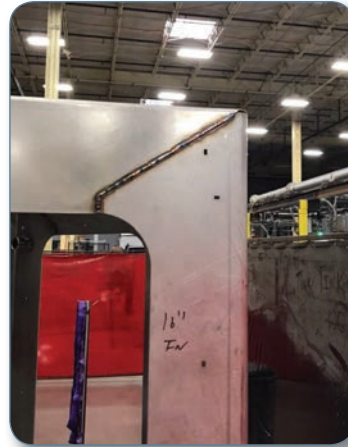
Left: Image of Glovebox Shell with Slots Cut, Middle and Right: Solidworks Image of Slot and Tab Fit Up
