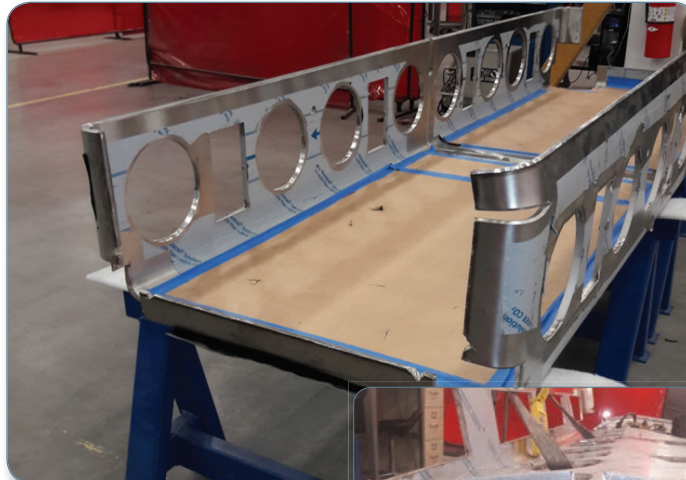
Examples of Relief Cuts from a 5/8-inch Thick Shell
